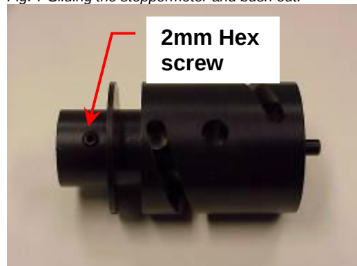
Fig. 8 Horizontal movement bush removed from the motor
