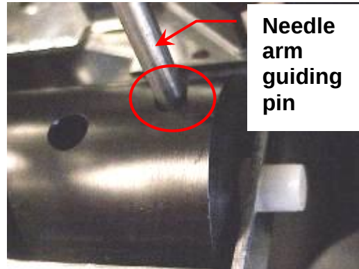
Fig. 12 Guiding pin of needle arm not correct at stop position of bush
