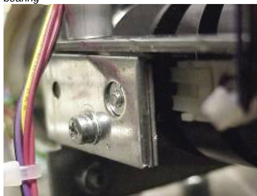
Fig. 10 Optical sensor flat assembled to frame
